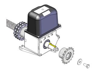
Attention! The drive-shaft and the driven system must be aligned.
