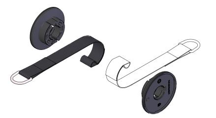
One or 2 belts can be mounted on each drum. Unscrew both bolts to take away the flanges. Slide the end of the belt over the bolt and refit the flanges and bolts. Apply a torque of approximately 6 Nm | 4.43 lbf to tighten the M5 bolts.
